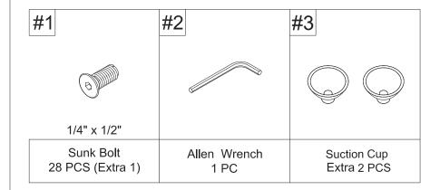
Step 1. Insert front rail (part C) and back rail (part D) into panels (parts A & B) using sunk bolts (part #1) and allen wrench (part #2).
